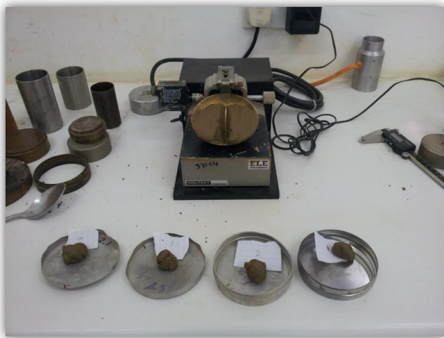
Fig. 14. Determining the Liquid Limit for the used Soil
