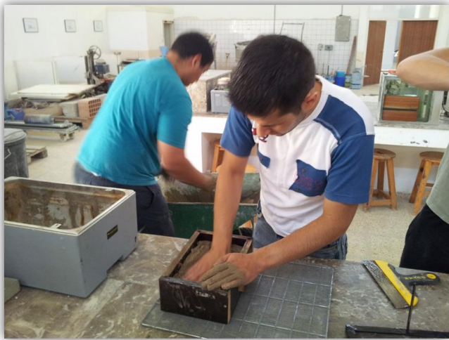
Fig. 10. Moulding the adobe into the wooden mould
