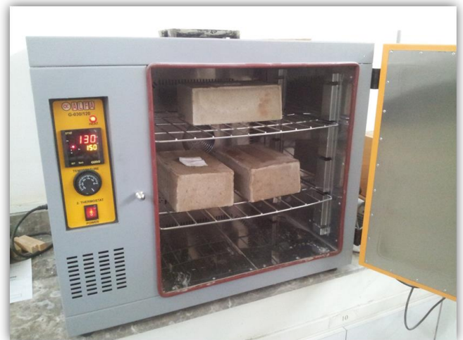
Fig. 13. Drying Process in the Oven at 150°C
